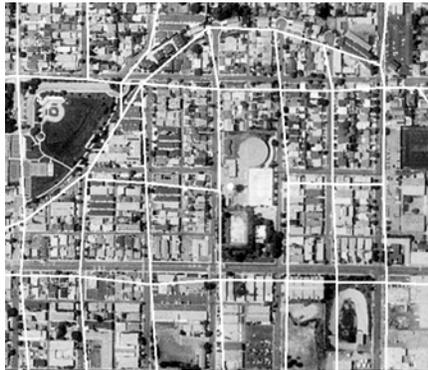
Figure 6. After applying conflation, utilizing VMF-filtered online data sources
