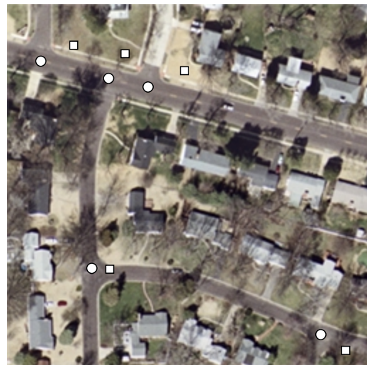
Figure 2.7: The intersections (rectangles) on road network data and the corresponding intersections (circles) on imagery
