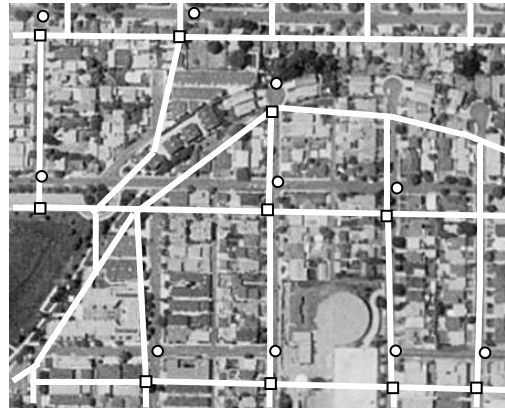
a) The original road network and detected control point pairs (one is marked by rectangle and the corresponding point is represented as circle)
