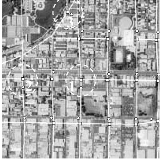
Figure 9 The intersections (rectangles) on road network data and the corresponding intersections (circles) on imagery (intersections 1, 2 and 3 are misidentified points).
