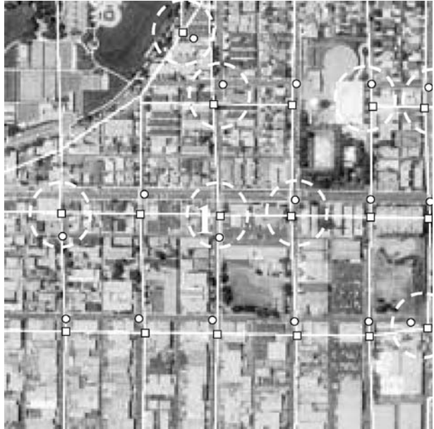
Figure 11 After applying VMF on Figure 10(a). The circles mark the control points categorized as outliers by VMF.
