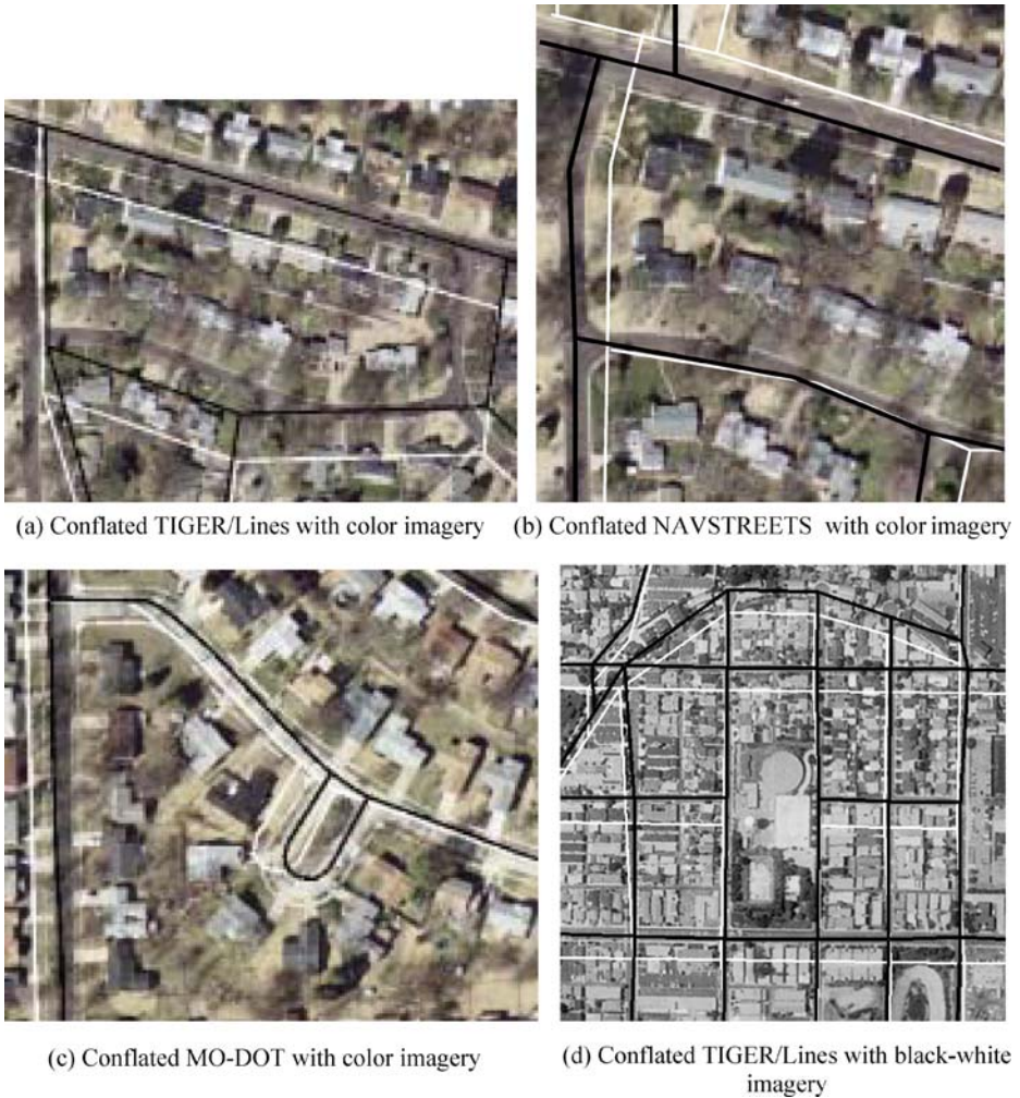
Figure 21 Vector-Imagery conflation (white lines: original road network; black lines: after applying conflation).
