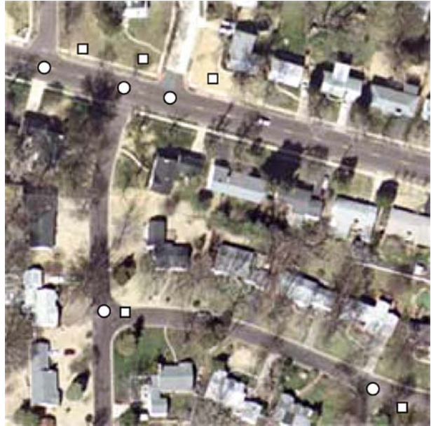
Figure 8 The intersections (rectangles) on road network data and the corresponding intersections (circles) on imagery.
