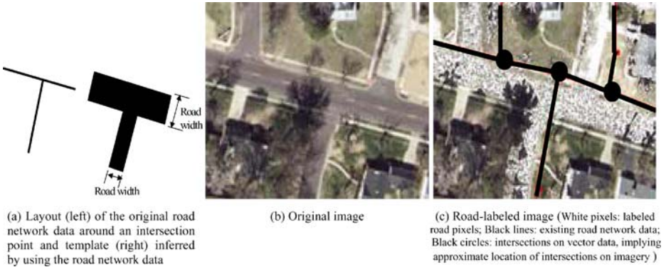
Figure 6 An example of the localized template matching.
