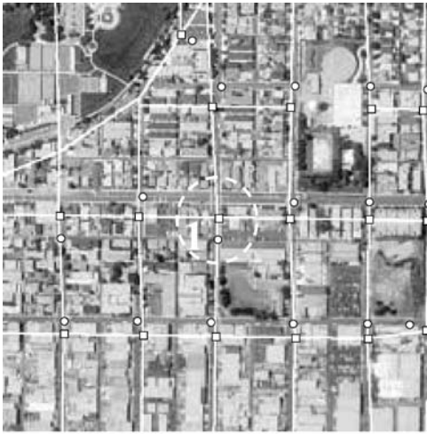
(a) The distribution of seventeen control point pairs (represented as rectangles and circles) in a small area centered at the control point 1
