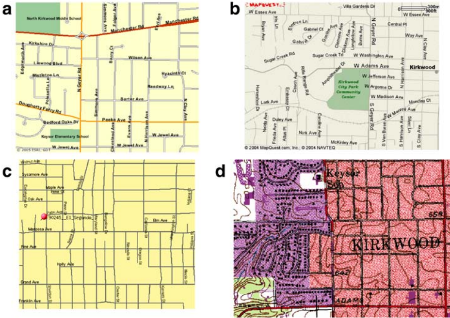
Fig. 15 Samples of different street maps used in the experiment. a An ESRI map with unknown map scale. b A MapQuest map with resolution 4.8 meters/pixel. c A TIGER map with resolution 4.17 meters/pixel. d A topographic map with resolution 2 meters/pixel
