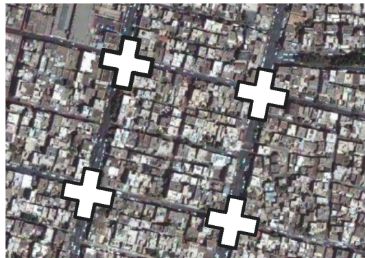
(c) Extracting roads from imagery using road-intersection templates extracted from a map
