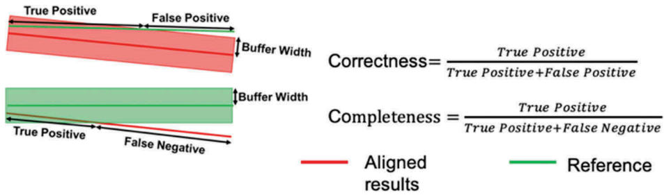
Figure 13. The illustration of correctness and completeness (the red line is the aligned result, and the green line is the reference.).
