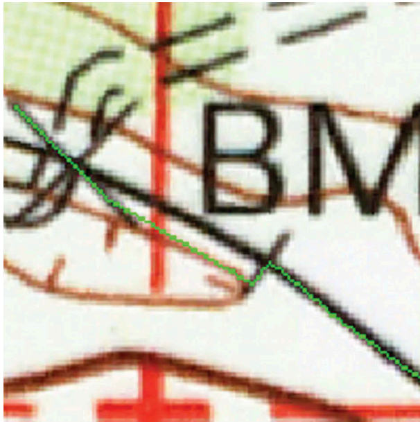
Figure 24. An example of the mis-aligned railroads where the green line is the output vector data from our algorithm.
