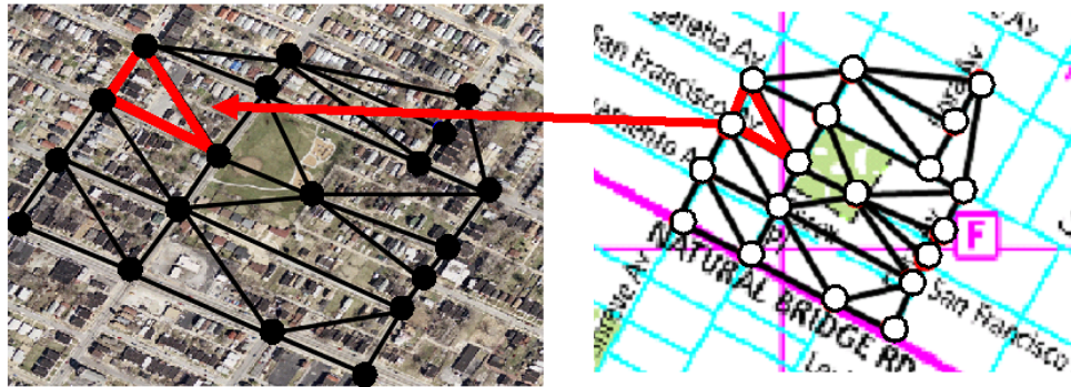
Figure 14. Partition each dataset into corresponding triangular regions based on the control point pairs (black points on the image and corresponding white points on the map)
