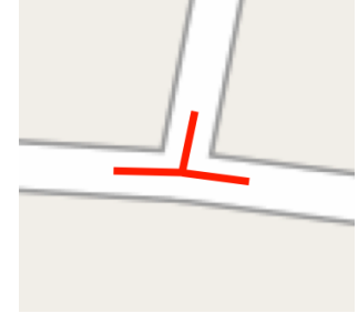
Figure 10. An example road-intersection template
