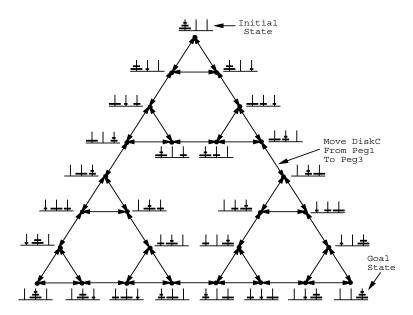
Figure 2: State Space for the Three-Disk Tower of Hanoi Puzzle
