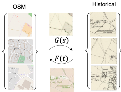
Figure 3: Illustration of CycleGAN. Generator G learns to convert OSM images to historical style and another generator F learns to convert the historical map images to the OSM style. During training, both generators are trained together with domain-specific discriminators. During synthetic data generation, only G will be used to synthesize historical map images from OSM.
