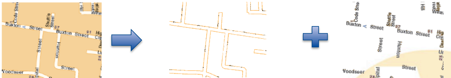
Extraction of road layers and text labels from raster map (Chiang et al. 2010)
