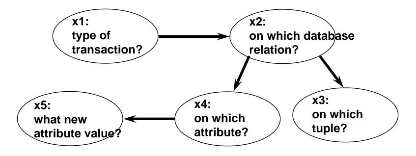
Bayesian network model of rule invalidating transactions Pr(t|d) = Pr(x1,x2,x3,x4,x5|d)= Pr(x1|d) Pr(x2|x3,d) Pr(x3|x2,d) Pr(x4|x2,d) Pr(x5|x4,d)
