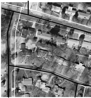
Figure 8: Vector-Imagery conflation (White lines: original road network; Black lines: after applying conflation using identified intersections)
