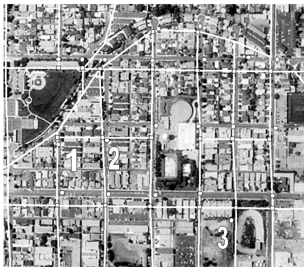
(a). The intersection points (rectangles) on vector data and the corresponding intersection points (circles) on imagery.
