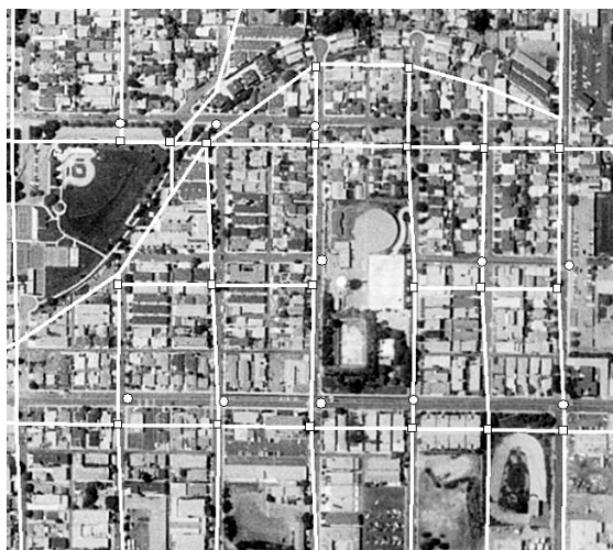
(c). The intersections left after applying vector median filter on Figure 7(a).
