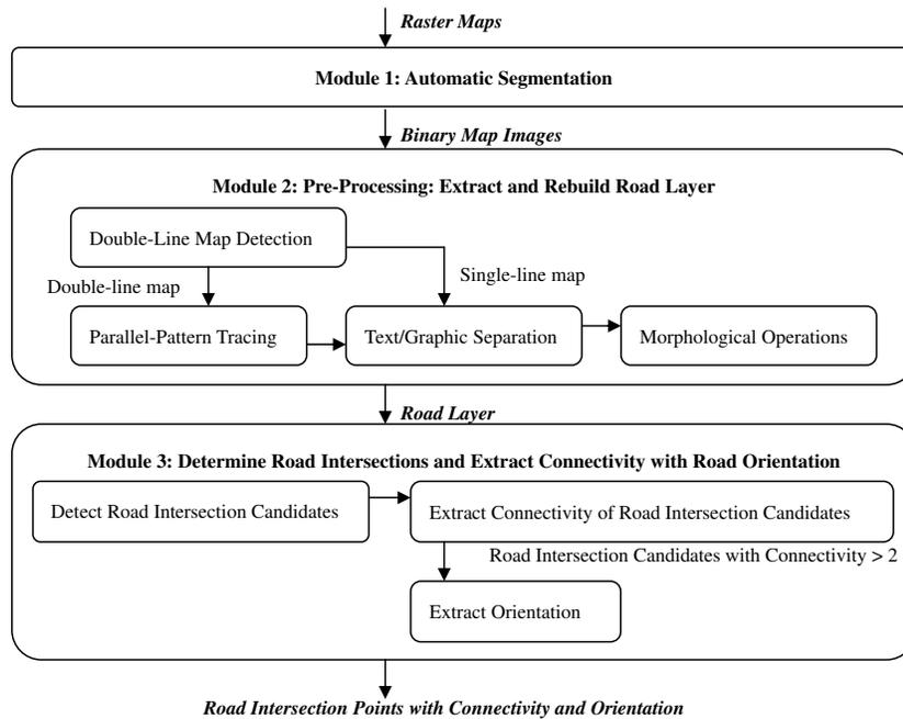
Figure 2: The overall approach to extract road intersections
