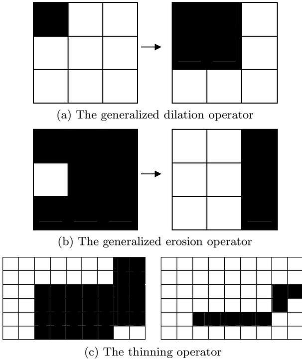
Figure 10: The morphological operators (black cells are foreground pixels)
