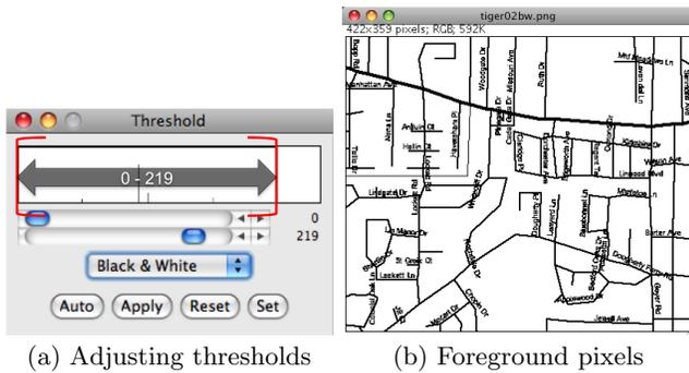
Figure 1: Adjusting thresholds in the grayscale histogram to extract foreground pixels from a TIGER/Line map
