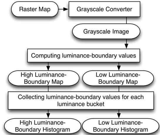
Figure 7: The approach to generate the high and low luminance-boundary histograms
