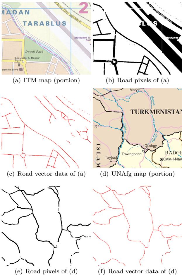
**Fig. 29** Examples of the road vectorization results on the ITM and UNAgf maps
