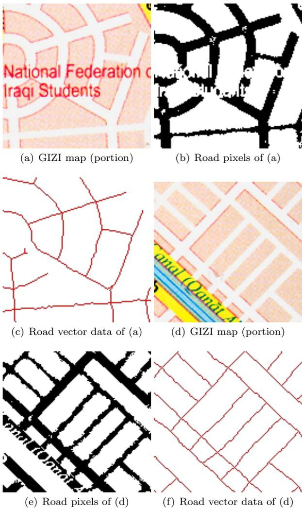
**Fig. 31** Examples of the road vectorization results on the GIZI map
