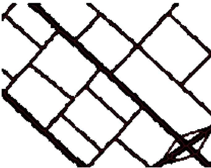
**Fig. 28** R2V results with manual image editing (red lines are the extracted road vector data and black pixels are the edited road area)
