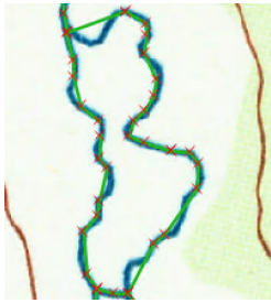
(a) An example of sharp turns (The vector data are in green. The red crosses are points in the vector data.)
