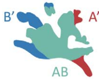
Fig. 5. Illustration of a geometry partitioning result for a polygon geometry: each color represents a different building block. A single building block may contain disconnected areas.
